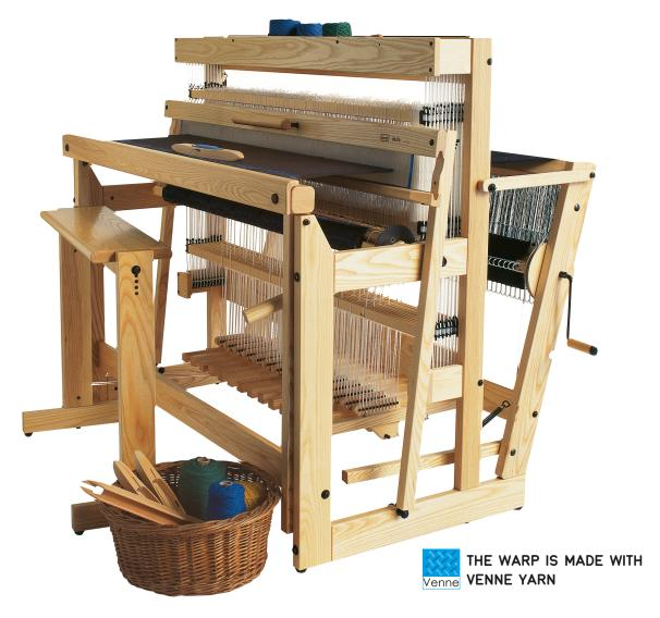
A comfortable and sturdy loom designed with all the innovative features, Delta utilizes the renowned Louët parallel counter march system and a floating breast beam, enhancing your weaving experience.
