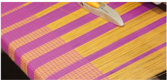
An ingenious spring system lifts all harnesses that aren't treadled down, ensuring equal tension on upper and lower shed. The cam system allows a weaver to effortlessly hold their shed open. The warp beam is equipped with a friction brake, allowing you to easily advance your fabric while
