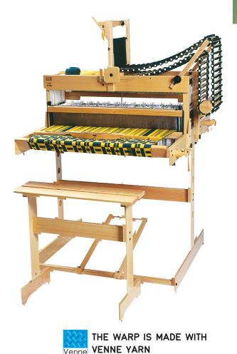
For a loom capable of complex weaving our Magic Dobby (MD) is also a very portable loom. Using the MD as a table loom, you open the shed, lifting the selected harnesses by the lever. If the loom is mounted on the included floor stand, you can open the shed by pushing the treadle. The front and rear sections fold up towards the castle, for easy storage or travel.
