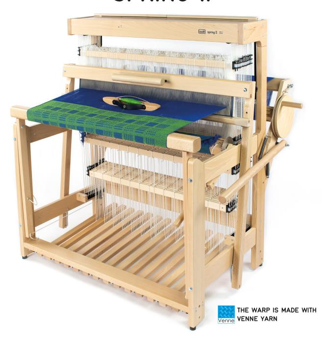
Spring, a counter march loom designed for versatility and precision, available in 90 cm (35 %") and 110 cm (43 ¼") weaving widths. Choose between eight or twelve harnesses to suit your weaving needs. Spring features an innovative parallel counter march system for harness action, along with a floating breast beam that allows you to easily control the tension of the warp. These advancements ensure that the loom meets the highest expectations of functionality and quality from weavers.
