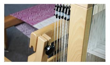
Changing or setting up tie-ups is a breeze with Spring; simply hook on the supplied Texsolv loop cords, which come pre-cut to the perfect length. The warp beam is equipped with a friction brake, allowing you to advance your fabric comfortably while seated at the loom. Plus, the beater with it's front handle is adjustable for both height and level, giving you greater control over your weaving.
