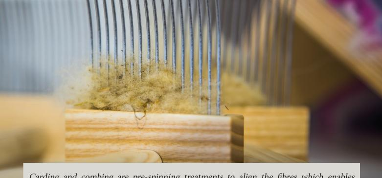
Carding and combing are pre-spinning treatments to align the fibres which enables you to spin fibres more easily. For the technique of felting or making woolen blankets, carding is essential. Combing straightens the fibres more than carding. This difference determines the character of the spun thread: worsted or woolen-spun.
