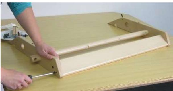
To assemble the back part of the David, use the warp beam supports, the back beam and the warp beam (one of the two round beams with a ratchet wheel).
