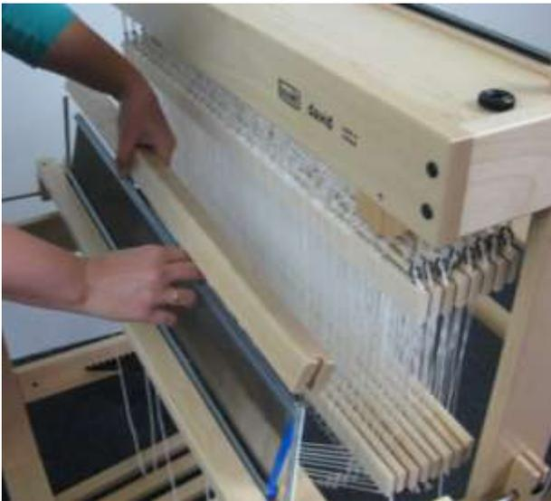
Position the reed and the upper reed holder in between the threaded rods and fasten the assembly with the knurled nuts.
