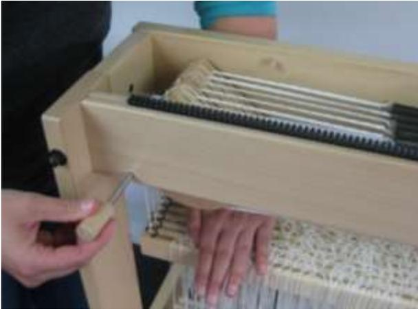
Remove the locking pin. It helps when you push the shafts a bit downwards.
