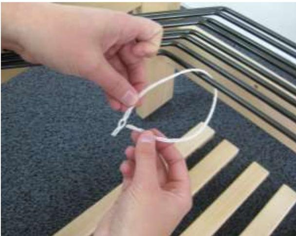
The tie-up cords for the treadles have already been cut to the correct lengths.
