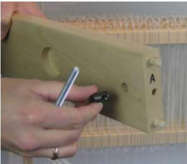
The uprights of the middle part are marked **A** and **B** at the location where they should be connected to the corresponding marked sides of the top side rails.
