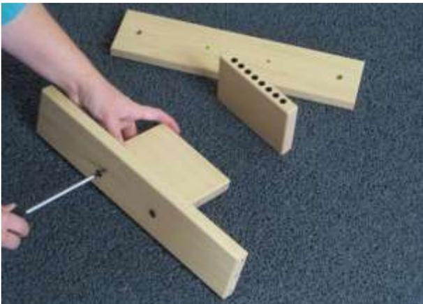
If your loom is a David 90, use the four 5x50 screws and attach the lam squares to the lower side rails at the same side where the holes for the barrel nuts are located.
