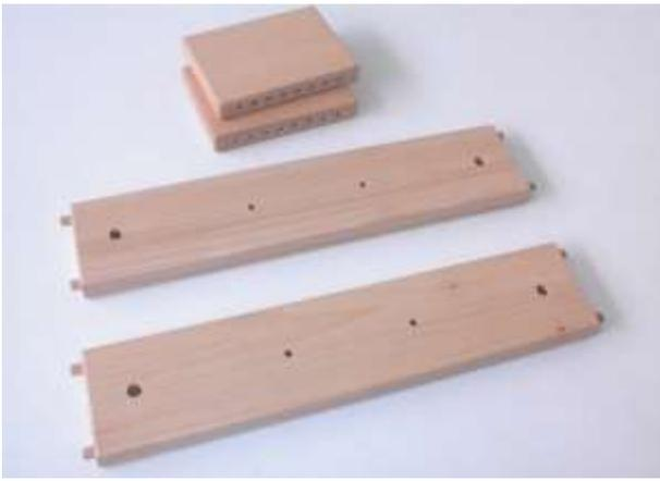
The picture on the left shows the lower side rails of the David 90 and the additional lam squares in which the nylon bearings are inserted.
