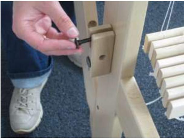
Slide the block with the two slots on the carriage bolt. Note that the oval hole faces the front of the loom. The second carriage bolt has to be plugged into the other slot and the other hole. After you've fastened the bolts with washers and wing nuts, mount the second block onto the post at the other side of the loom.
