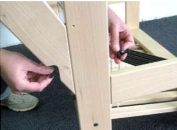
Insert the threaded ends into the holes through the uprights and warp beam supports, slide on the washers and fasten the wing nuts.
