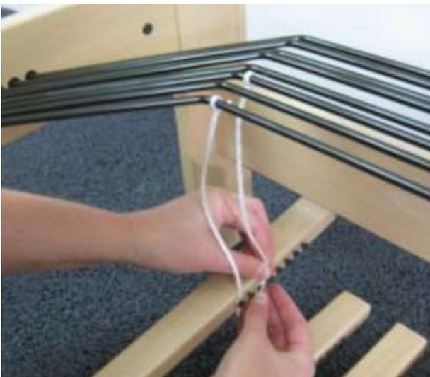
Hook the other end of the cord to the corresponding screw head of the treadle.
