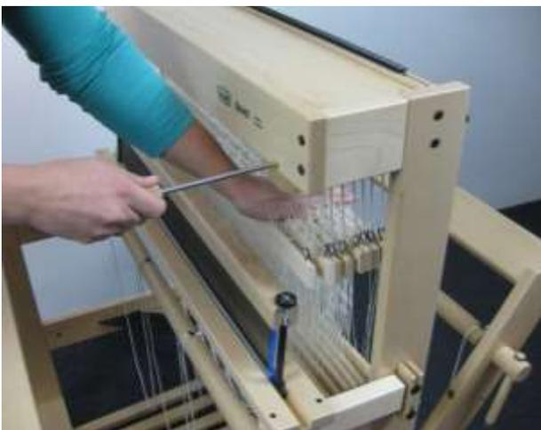
If you want to add heddles or to remove heddles from a shaft, you have to unhook cords from the shaft bars. This is easier after you have blocked the system by inserting the locking pen through the wooden discs. In this situation the springs give no tension on the system.
