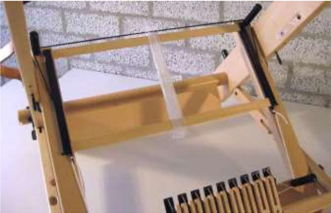
Adjust the position of the shaft as shown on the picture by changing the length of the nylon cord. The distance between the elastic cord and the bottom of the shaft should be about 8 mm (5/16"). Later on we can adjust the shafts more precisely.
