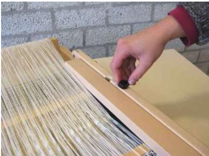
Lock the Jane in its folded situation by screwing the black knobs onto the threaded ends located in the hole in the beater supports.
