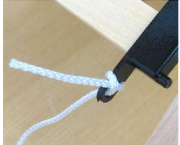
Attach the cord to the eye of the sides of a shaft. Use the knot shown in the picture: Insert the cord from the inside, where the eye has a sharp edge, so the cord crosses itself at the outside.
