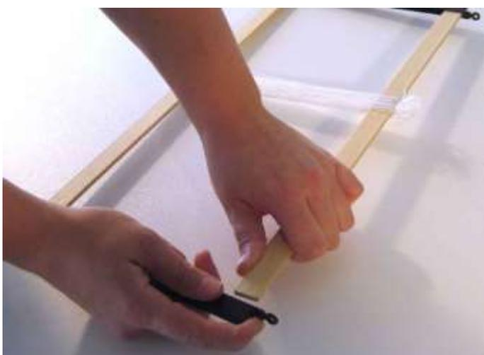
Install the other shaft side and make sure that the eyes at the end of both shaft sides point in the same direction.
