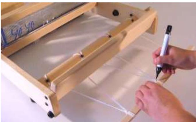
Tighten the loops by pulling on the apron bar.
