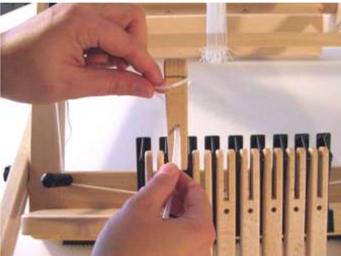
Now attach a second shaft cord to the next toggle and lead it through in between the hinges and the rollers.
