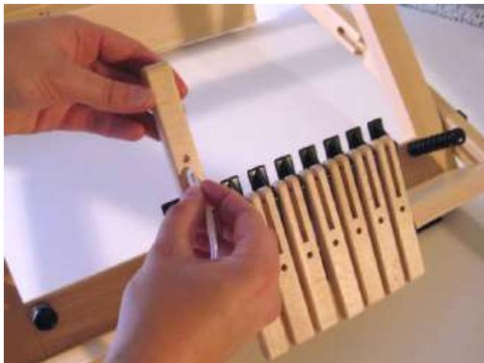
A shaft cord has to be attached to the toggles. Start with the toggle for the eighth shaft; when the loom is in the upside down position shown in the picture, it is the one at the left.
