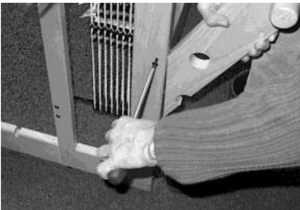
Secure the polyurethane dowels by screwing the screws completely into the uprights, while holding the back part in a position that let the dowel in completely.
