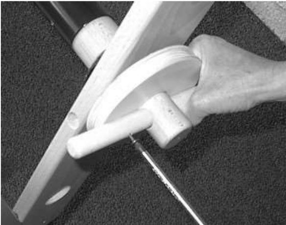
Slide the brake disc over the wooden end of the warp beam and fasten it with the dowel and the two screws 4 x 35 mm.
