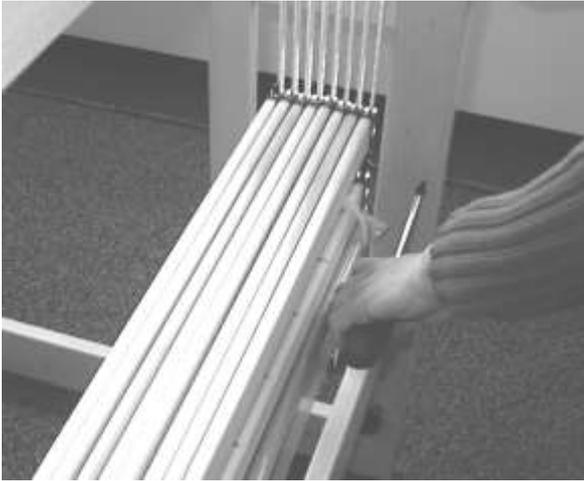
Screw the two 4 x 25 mm screws a few turns into the main uprights at the level of the holes in where the back part will be attached. The uprights are identical so you will find one pilot hole at the inside and one at the outside of the loom.
