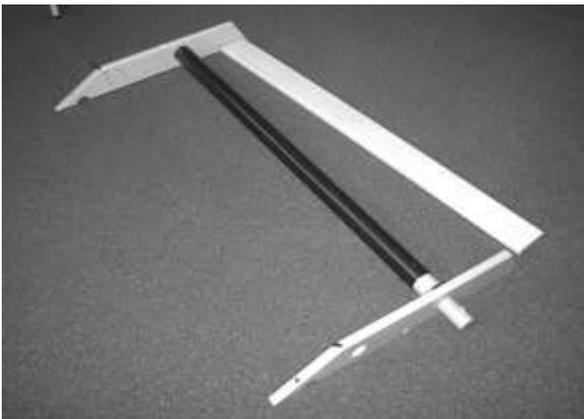
Take the warp beam, the back beam and the two warp beam supports and place them together as shown on the picture. Insert the shaft of the warp beam through the right support and slide the left support onto the other end of the warp beam.
