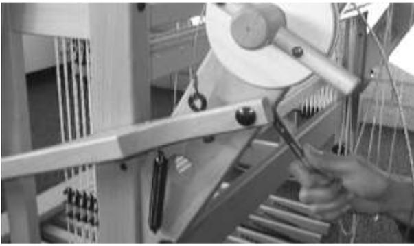
Tap the carriage bolt into the hole of the lever from the side that is curved and slip on four washers and the bushing.
