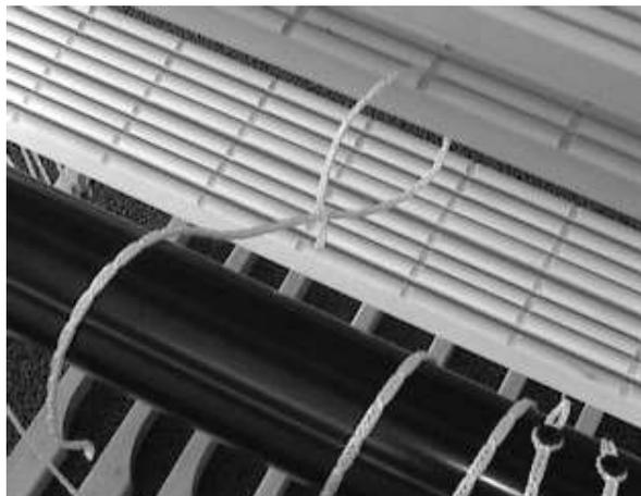
First make the tie-ups to the upper lams. Loop the cord around the lam and pass one end through the last loop in the other end. Tighten it after the cord is positioned in the groove in the lam, right above the treadle to be tied.
