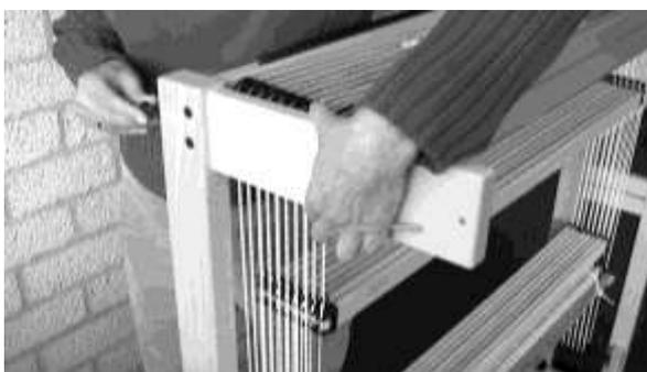
Insert the barrel nut into the new top side piece and assemble it in the reversed sequence, the barrel nut facing the inside.
