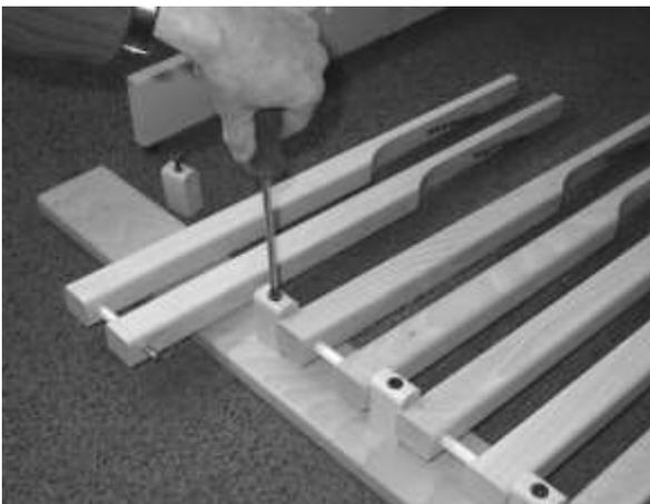
Place the foot rail upside down (pilot holes up) on the floor in front of the loom.
