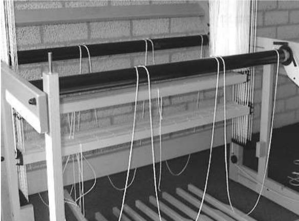
Attach the beam cords onto the screw heads of the cloth beam and the warp beam.
