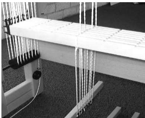
The cords should be tied to the screw heads on a treadle in a sequence, corresponding to the shafts.
