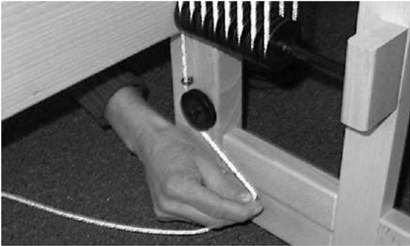
Bring the attached cords down through the screw eyes at the bottom of the main upright and lead them along the roller.
