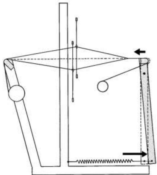
The moving breast beam is held by springs, adjustable to give your warp the tension needed for your project. Besides improvement of the shed and protection of the warp, the springs guarantee exactly the same warp tension each time you have to advance the fabric.
