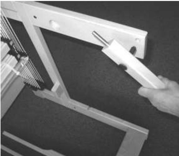
Take the wooden posts, recognizable for the steel rod at the end. These floating arms will hold the moving breast beam.
