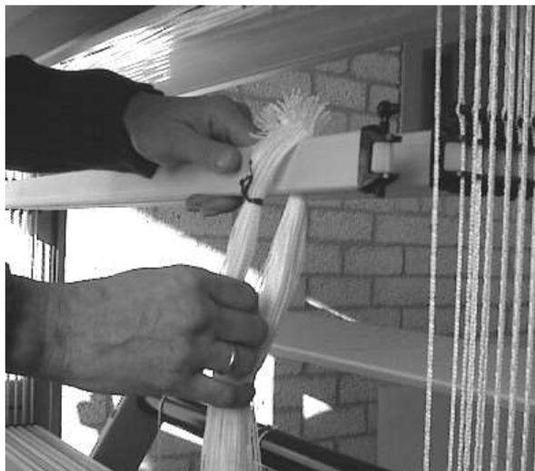
If you need to add heddles to a shaft, pull the hook that connects the upper shaft bar to the cord, out of its cord loop. Slip over a bundle of heddles and push the hook back into the same loop again. Repeat this with the lower shaft bar, but untie the bundle before you attach the lower bar into the cord again.
