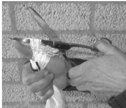
If you need to remove heddles from a shaft, first tie them as they were originally. Use a pair of sharp scissors to cut the heddles apart.
