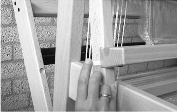
The upright that leaves the buffer last when you pull the beater, is the one that needs one or more cardboard strips in its slit connection with the lower reed holder.
