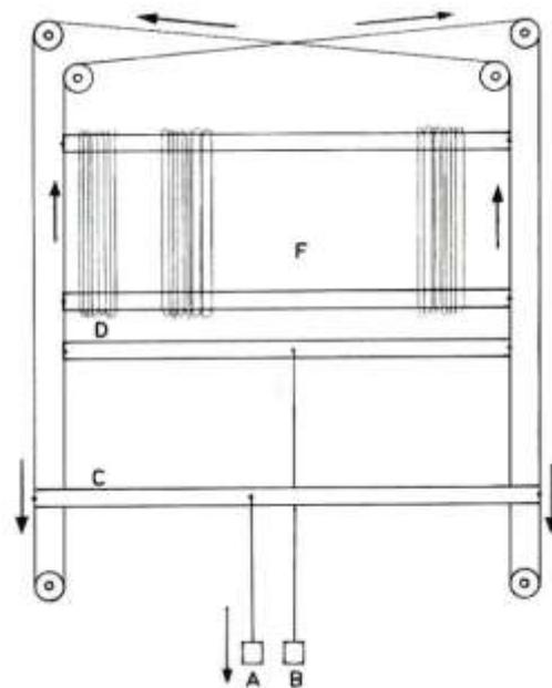
3. Shaft bars and lams cannot slant. Their ends are fixed to the cord and when the cord moves, all parts of the cord have to move the same distance.
