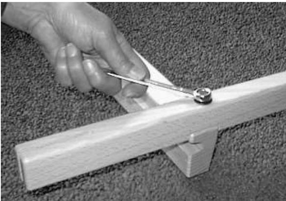
Connect the lower reed holder (the one with the slanted side) to the uprights: Place the barrel nut into the hole on the end of the lower reed tray. Slide the upright with the notch over the lower reed tray. Place the bolt with washer in the hole and screw it into the barrel nut. Tighten the bolt and, in the same way, assemble the other upright on the other side of the reed holder.
